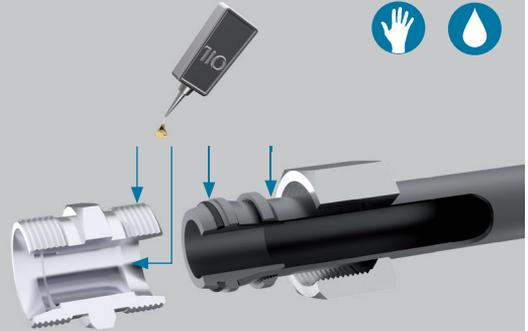
**4.2** Insert the pre-assembled tube end into the cone of the coupling connecting piece at a straight angle.
