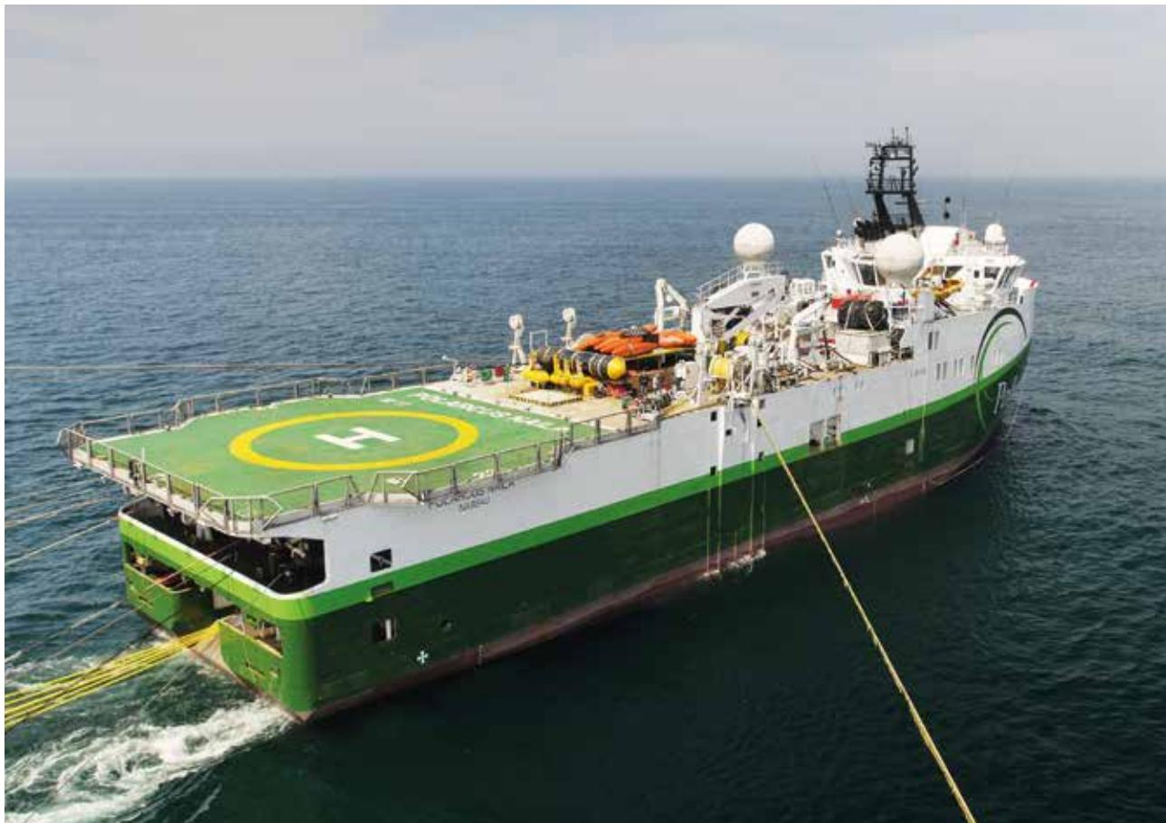
Seismic vessels have special compressors for feeding the air guns with pressure capacity of up to 2000 psi. These compressors are capable of supplying high pressure air to the air guns continuously over a very long period of time. Once the line is completed, the vessel will maneuver to a new starting point as advised by the navigators and the whole process repeats. The ideal speed of the vessel while acquiring data is kept between 2 and 5 knots.
