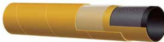
**Compressed air 20 bar (300 psi) - Heavy Duty****Tube:** Black SBR/NBR - oil mist resistant.**Reinforcement:** High tensile textile cords.**Cover:** Yellow SBR - abrasion and ozone resistant.**Application:** Compressed air designed for heavy duty applications.**Safety factor:** ≤ 51 mm 3:1 ≥ 63 mm 2,5:1**Temperature:** -30 °C +80 °C (-22 °F +176 °F)
