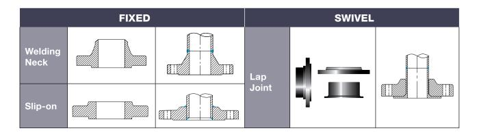
ALFAGOMMA offers a complete range of flange faces for built-in and swaged fittings:
