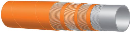
**Rig supply soft wall - Potable water 20 bar (300 psi)****FDA****Tube:** white NR.**Reinforcement:** high tensile textile cords.**Cover:** orange NBR/PVC - abrasion, ozone and hydrocarbon resistant.**Application:** potable water transfer from supply vessels to offshore platforms.
