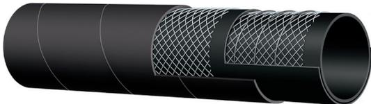
**Fuel-oil S&D 20 bar (300 psi)****Tube:** black conductive NBR**Reinforcement:** high tensile textile cords with embedded steel helix wire - antistatic wire**Cover:** black CR - abrasion, ozone and hydrocarbon resistant**Application:** fuel, oil and liquid mud transfer between supply vessels and offshore platforms.
