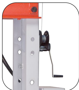
Winch provides easy positioning of press bed
