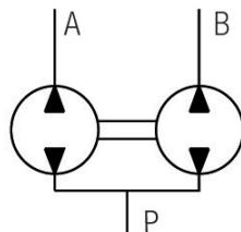
**Construction:** Rotating flow divider, gear type
