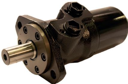
**Construction:** Gerotor type design**Shaft:** Straight key 25mm**Flange:** SAE A-2**Ports:** 1/2" BSPP**Application:** Conveyors, food industries, metal working machines, road building machines, mining machinery, special vehicles**General:** Shaft seal 150 bar**Benefits:** Low speed, high torque, high starting torque, high efficiency.**Manufacturer:** M+S
