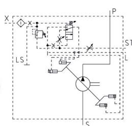
**Construction:** Single or double piston pumps with variable displacement. Regulator: Load-sensing, adjustable power limitation
