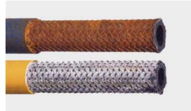
The advantages of the zinc-plated steel braids become obvious when effecting a salt water test. The Galvanator has been soaked in a 5% salt water solution at 45° for 48 hours.
