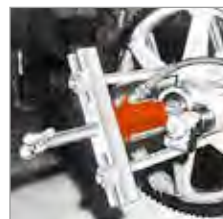
Hydraulically powered Bi-Directional™ Puller removes drive wheel. Pulling attachment is used to provide gripping surface.
