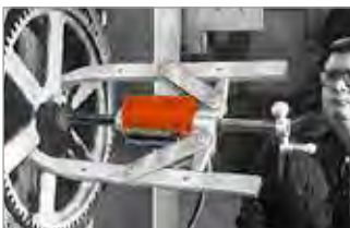
2-jaw puller reaches through spokes of gear to grip hub. Hand pump supplies hydraulic power.
