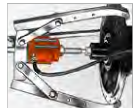
3-jaw puller provides grip while hydraulic hand pump provides power to push shaft from housing. Shaft protector is used on end of puller screw.
