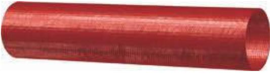
**Water discharge - PVC - Lay flat - Heavy duty****Tube:** Red PVC.**Reinforcement:** high tensile textile cords.**Cover:** red PVC - abrasion and ozone resistant.**Application:** lay flat water discharge.**Temperature:** -10 °C +60 °C (+14 °F +140 °F)
