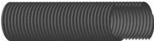
**Air ducting - PVC - Steel helix****Construction:** black PVC**Reinforcement:** pvc coated steel helix wire**Application:** air, gas, fumes extraction. Air conditioning-ventilation.**Temperature:** -10 °C +60 °C (+14 °F +140 °F)
