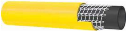
**Antitorsion garden irrigation - PVC****Tube:** black PVC.**Reinforcement:** high tensile textile cords.**Cover:** yellow PVC.**Application:** water delivery.**Temperature:** -10 °C +60 °C (+14 °F +140 °F)
