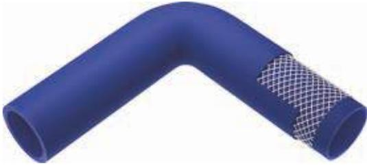
**Radiator - Silicone - 90° Elbow****Tube:** blue silicone**Reinforcement:** high tensile textile cords.**Cover:** blue silicone**Application:** radiator.**Temperature:** -56 °C +177 °C (-69 °F +350 °F)
