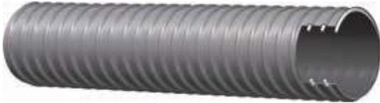
**Air ducting****Construction:** grey PVC - abrasion and ozone resistant.**Reinforcement:** white shock resistant rigid PVC.**Application:** air, gas, fumes extraction. Air conditioning-ventilation.**Temperature:** -10 °C +60 °C (+14 °F +140 °F)
