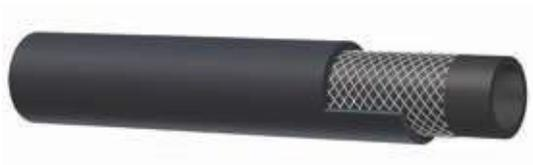
**Breathing air****EN 14593 - EN 14594****Tube:** black antistatic NBR.**Reinforcement:** high tensile textile cords.**Cover:** black NBR/PVC with green stripe - abrasion and ozone resistant.**Application:** breathing air.**Temperature:** -30 °C +100 °C (-22 °F +212 °F)
