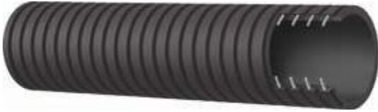
**Fuel-oil S&D - Square corrugated - Extra flexible****Tube:** black NBR**Reinforcement:** high tensile textile cords with embedded steel helix wire**Cover:** black CR - square corrugated, abrasion, ozone and hydrocarbon resistant**Application:** fuel and oil suction and delivery. Specially designed for tank truck and general industrial applications. Special square corrugated construction for maximum flexibility.**Temperature:** -25 °C +100 °C (-13 °F +212 °F) mm
