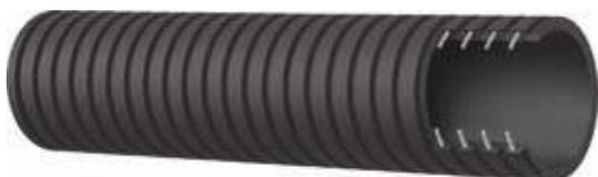
**Radiator S&D 6 bar (90 psi)****Tube:** black EPDM**Reinforcement:** high tensile textile cords with embedded steel helix wire**Cover:** black CR - square corrugated, abrasion, ozone and hydrocarbon resistant**Application:** general purpose-hot water. Specially designed for automotive heating systems. Special square corrugated construction for maximum flexibility.**Temperature:** -40 °C +120 °C (-40 °F +248 °F) mm
